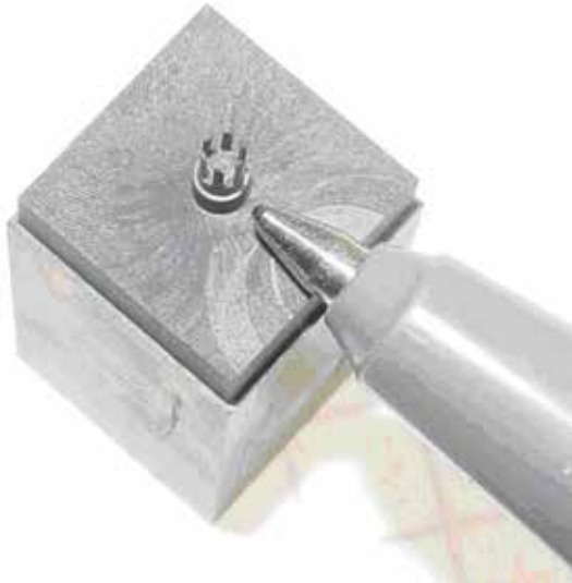
Figure 4 - Fine electrode detail increases the importance of a quality material.
