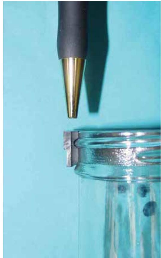
*Insert with optimal design will encapsulate thread without contact. Support is provided under thread during bottle removal.*
