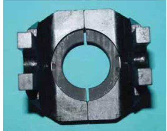
*Holder with insert designed to allow kerf. When installed in a POCO® holder, true diameters are achieved.*
